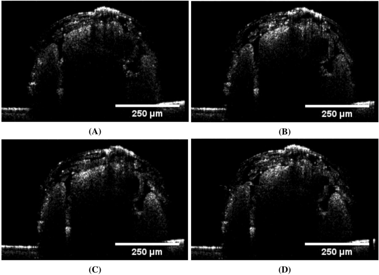
**Fig 12** B-scan-OCT images of *in-vivo Drosophila* with focus at -1 (A), 0 (B), and 1 (C) covering a total range of 1 mm axial range measured in air. Final image (D) is synthesized through extraction of in-focus regions from a stack of images acquired with focus shifted incrementally.
