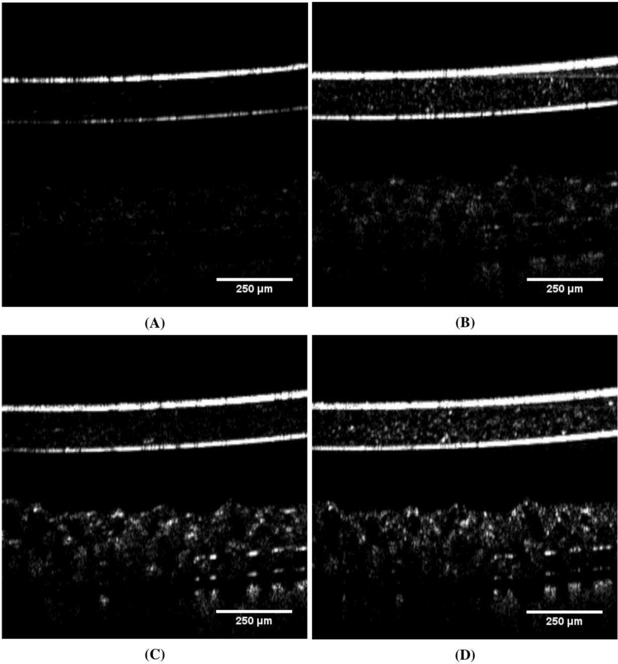
**Fig 11** OCT B-scan images of an infra-red card, with focus set to -1.5 (A), 0 (B), and 1.5 (C) covering a range of 0.75 mm. The final image (D) is the composite Gabor image.
