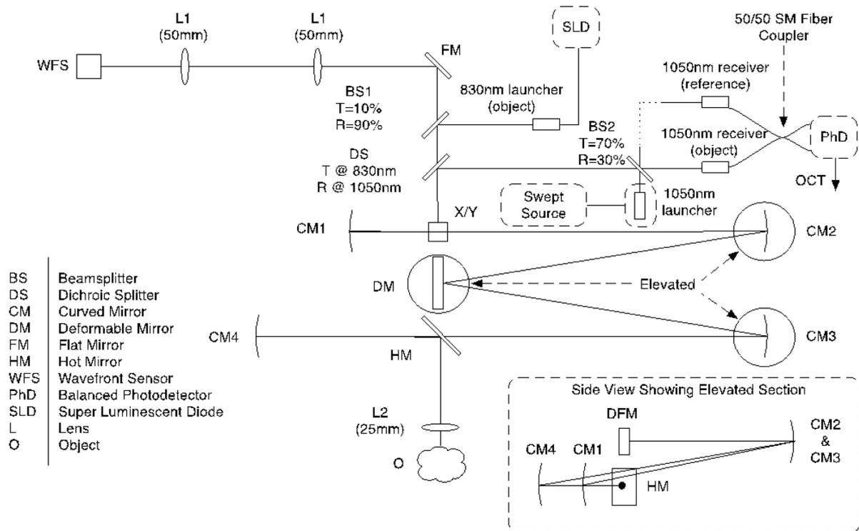
**Fig 1** Schematic of the AO/SS-OCT system with imaging at 1060 nm and wavefront sensing plus confocal microscopy at 830 nm.
