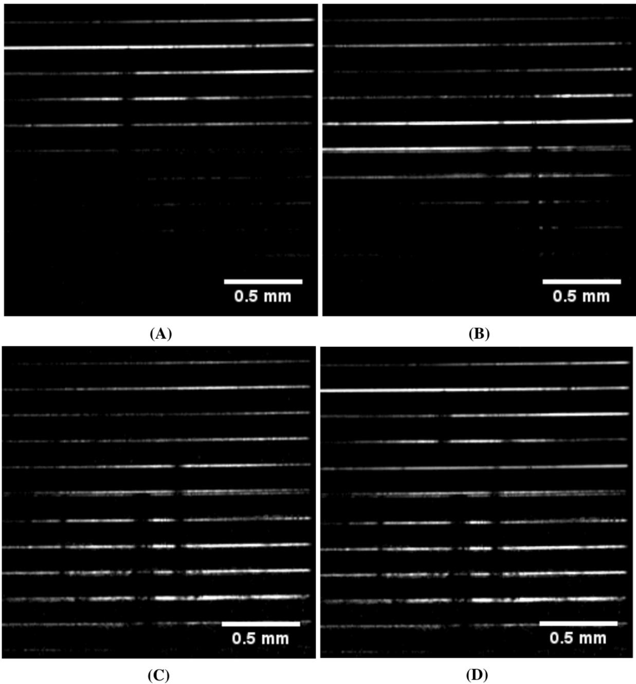
**Fig 10** Images acquired of a phantom constructed from ten 0.17 mm thick glass slides (bound top and bottom with sellotape of similar thickness) with focus set to -4 (A), 0 (B) and 4 (C) covering a total range of 2 mm. Final image (D) is synthesized through extraction of in-focus regions from a stack of images acquired with focus shifted incrementally.
