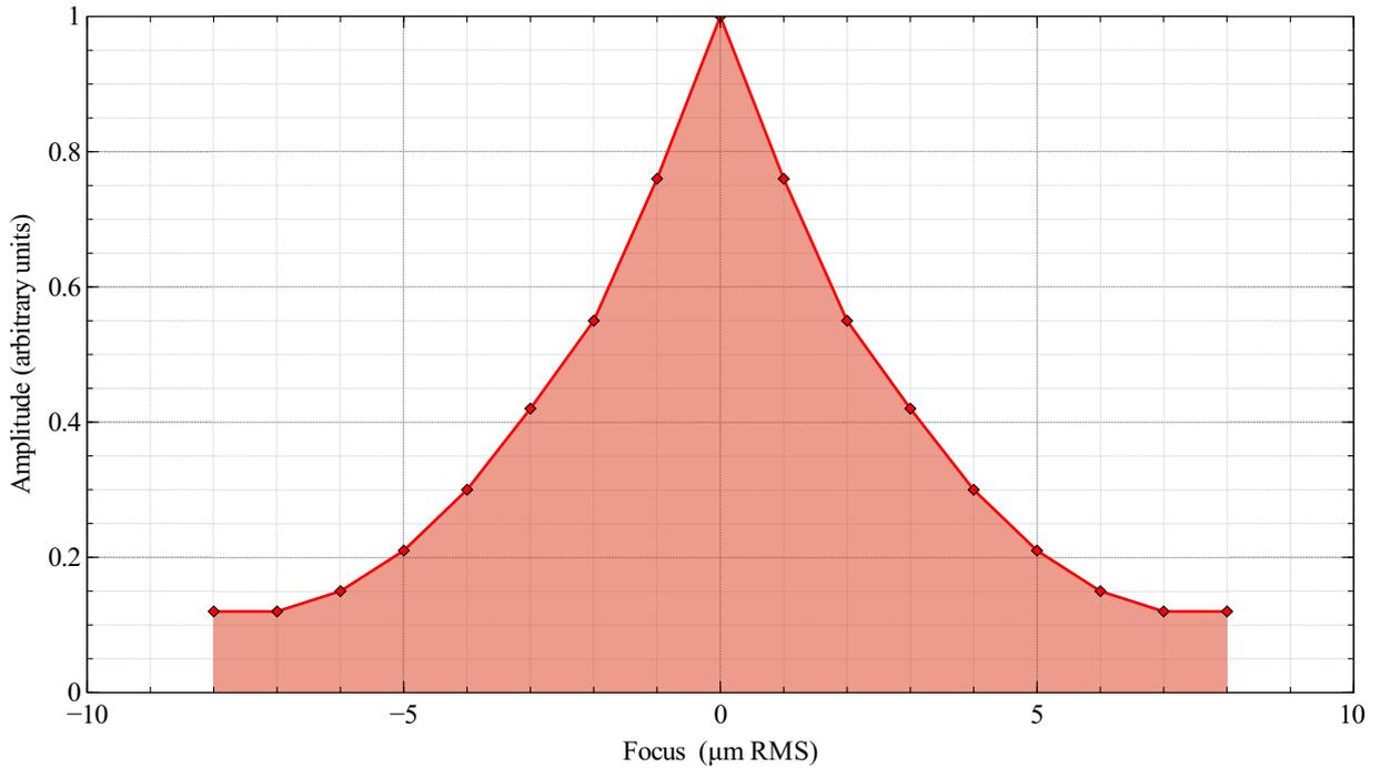
**Fig 3** Chart showing decay in signal intensity with added focus
