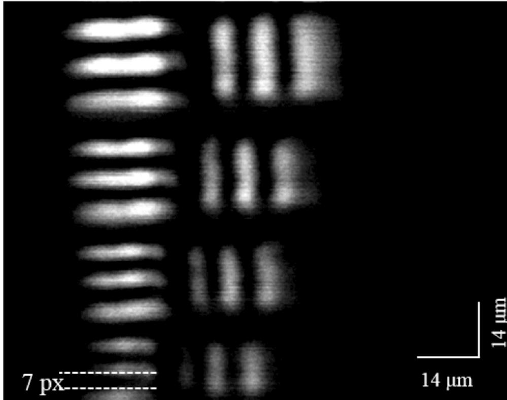
**Fig 4** High contrast confocal image of the USAF target showing the smallest  $2 \mu\text{m}$  bars at the bottom. Two sets of three bars are shown oriented horizontally and vertically. Image size is  $250 \times 250$  pixels covering an actual area of  $70 \times 70 \mu\text{m}^2$  on the target.
