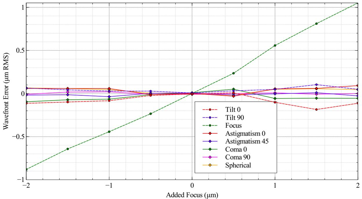
**Fig 8** Effect of focus manipulation on defocus aberration (green) and on seven other high-order aberrations (according to colour in the inset).
