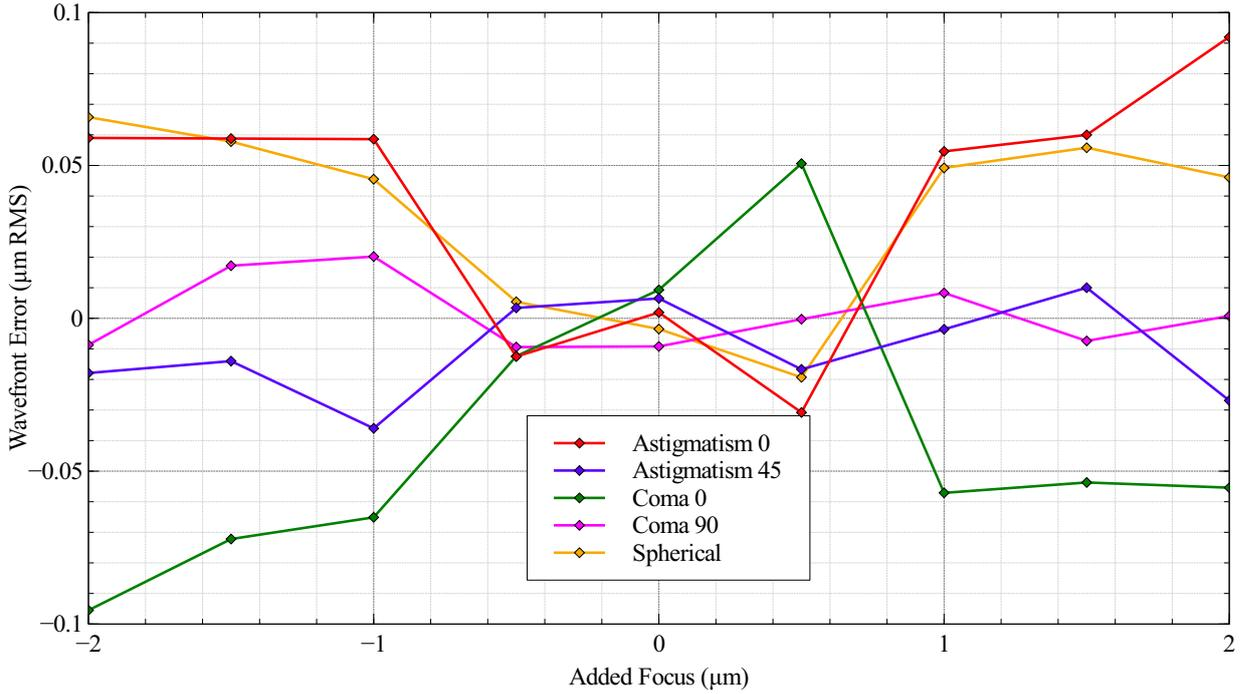
**Fig 9** Magnified view of WFS RMS error showing effect of focus on wavefront excluding tilts and focus aberrations.
