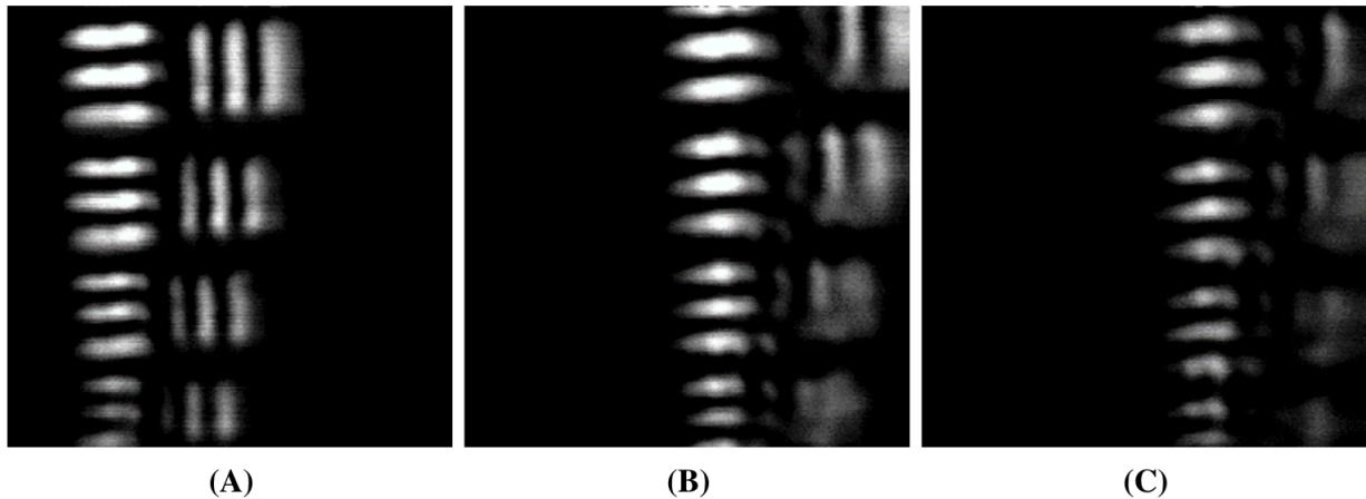
**Fig 6** Images of the USAF target obtained using the DM deformed to create 3  $\mu\text{m}$  (B) and 4  $\mu\text{m}$  (C) RMS defocus, with the original 0  $\mu\text{m}$  focus image (A) for comparison.
