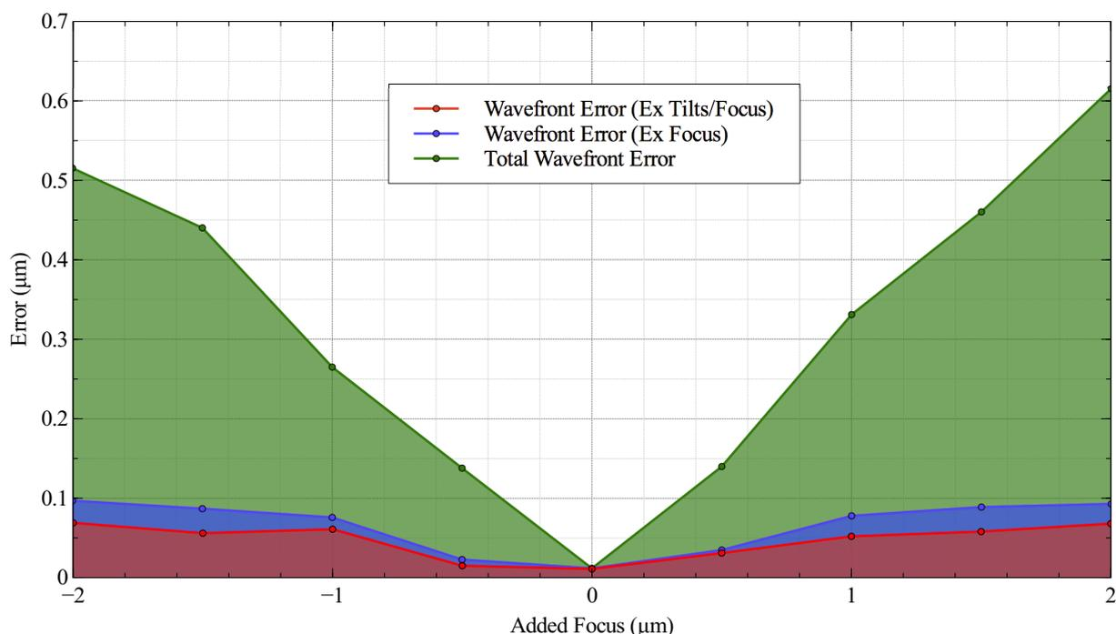
**Fig 7** RMS wavefront error as focus is manipulated. Total error: green region. Error excluding focus: blue region. Error excluding tilts and focus: red region.
