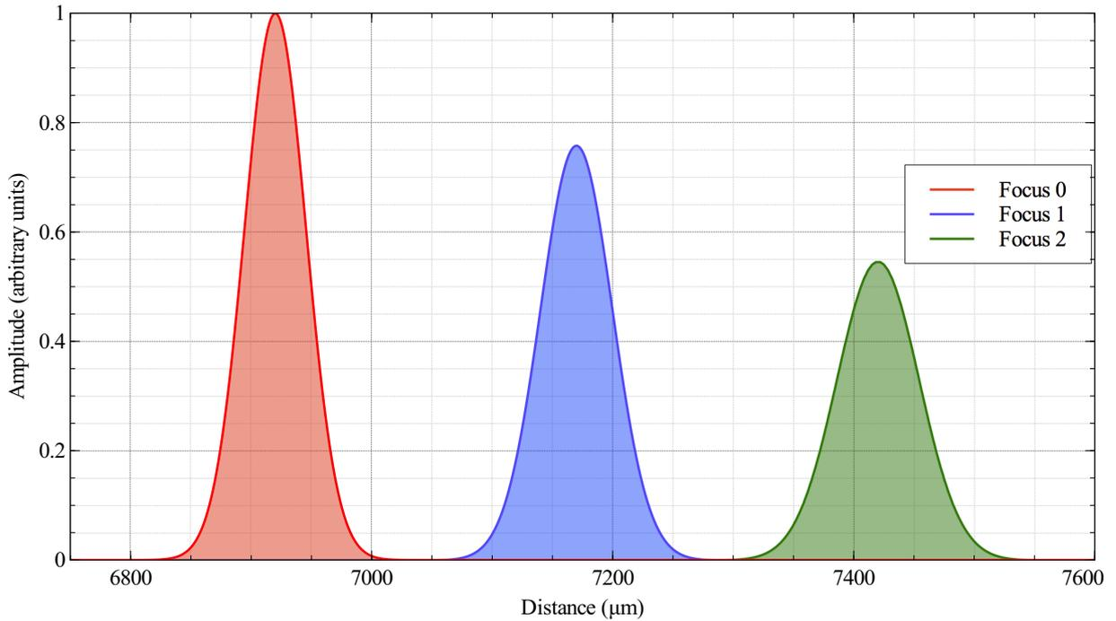
**Fig 2** Chart showing how the confocal profile shifts in depth and changes shape as we add 1 and 2  $\mu\text{m}$  RMS focus.
